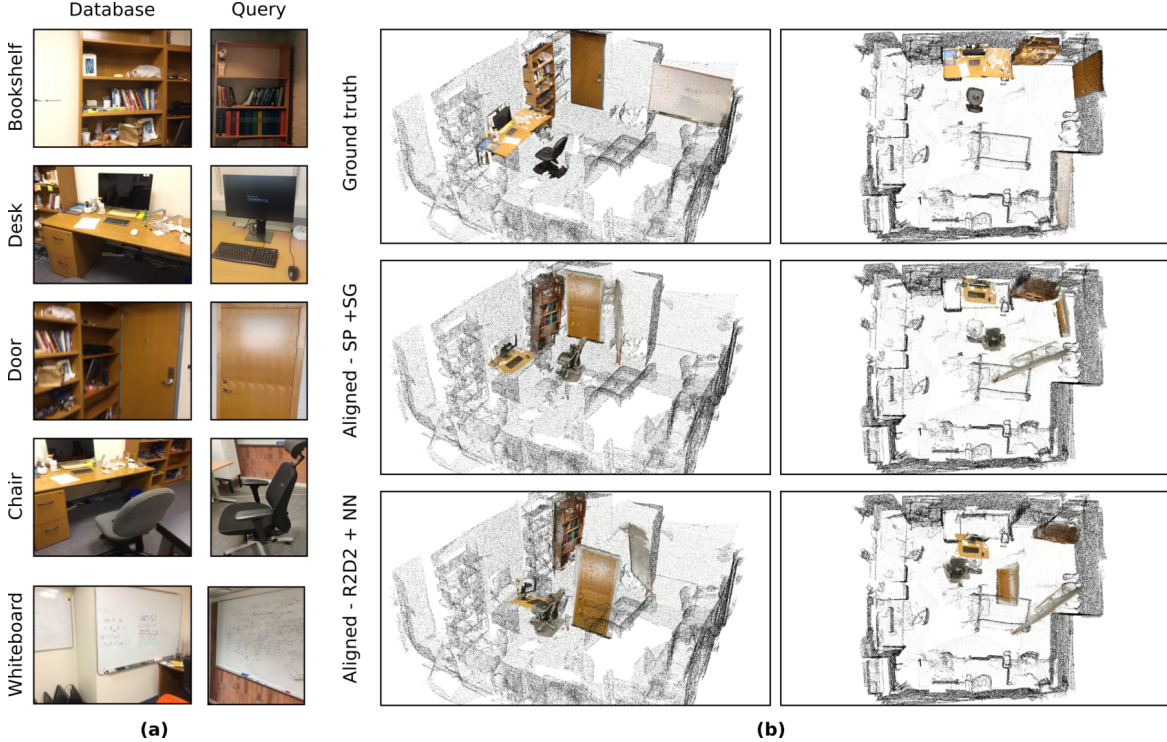
Figure 5. (a) Example images from ScanNet-Office-Scene and corresponding objects in Office-Objects . (b) Qualitative results for aligning generic office objects in ScanNet [8] scene0040 , using Superpoint+Superglue and R2D2+NN.
