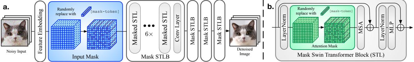
Figure 4. The transformer architecture of our proposed masked image training. We make a minimal change to the original SwinIR architecture – the **input mask** operation and the **attention masks**. Other micro-designs are not essentially different from other Transformers.
