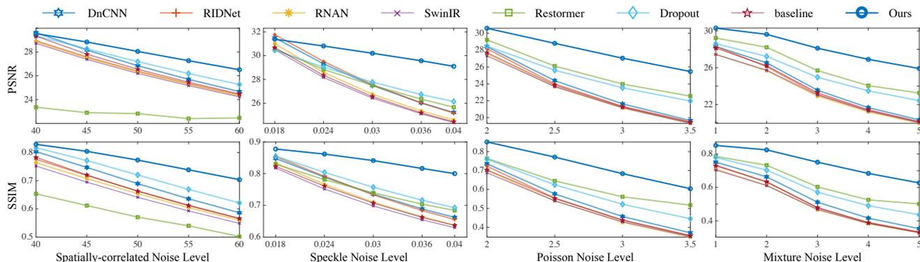
Figure 11. Performance comparisons on four noise types with different levels on the Kodak24 dataset [26]. All models are trained only on Gaussian noise. Our masked training approach demonstrates good generalization performance across different noise types. We involve multiple types and levels of noise in testing, the results cannot be shown here. More results are shown in the supplementary material.
