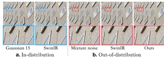
Figure 1. We illustrate the generalization problem of denoising networks. We train a SwinIR model on Gaussian noise with  $\sigma = 15$ . When tested on the same noise, SwinIR demonstrates outstanding performance. However, when applied to out-of-distribution noise, e.g., the mixture of various noise, SwinIR suffers from a huge performance drop. The model trained by the proposed *masked training* method maintains a reasonable denoising effect, despite also being trained on Gaussian noise.
