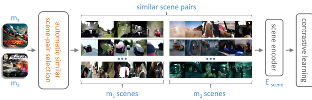
Figure 3. Contrastive Scene Representation Learning – Given a pair of similar movies \mathbf{m}_1 and \mathbf{m}_2 as determined by \mathcal{S} , we use a set of pre-processing operations (as shown in Figure 2) to select similar scene-pairs (see supplementary material for more examples). This process is applied to all similar movie-pairs to get a set of paired scenes that is used for scene-level contrastive learning.
