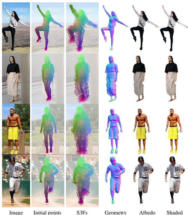
Figure 4. Output of S3F. Given an input image (first col.) and GHUM pose estimates (second col.), S3F displaces points efficiently to cover relevant features from the image (third col.). Displaced points cover areas that not necessarily belong to the foreground, but tend to represent loose clothing ( e.g. hair and loose clothing in first and second examples respectively). This coverage and the efficient feature retrieval allows to correct potential errors in the body such as the feet in the first two examples or the overall body orientation in the third row. Zoom-in recommended.
