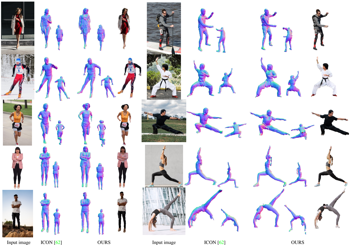
Figure 3. Qualitative 3D human reconstruction comparisons against the SOTA method ICON [62] for complex body poses. Images on the right column feature challenging poses and viewpoints. Notice the additional detail provided by our method, especially for hair and faces. We additionally recover per-vertex albedo (not shown) and shaded color. See Sup. Mat. for more examples and failure cases.
