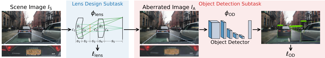
Figure 2. Overview of our joint design approach. To tackle the lens design and OD subtasks jointly rather than in isolation, we simulate realistic aberrations on the dataset images before they enter the object detector. The lens parameters \phi_{\text{lens}} (with curvatures c , spacings s , and glass variables g ) are optimized both on a loss \ell_{\text{lens}} , which targets optical performance and geometrical constraints via exact ray tracing, and on the OD loss \ell_{\text{OD}} . The object detector parameters \phi_{\text{OD}} are trained concurrently to minimize \ell_{\text{OD}} while adjusting to the lens aberrations.
