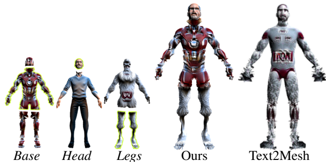
Figure 8. Controlled stylization. Given three different stylizations of the same object, we use 3D Highlighter to select different regions and combine them together (Ours). Attempting to achieve this composition with a holistic approach leads to an undesirable result (Text2Mesh [25]).
