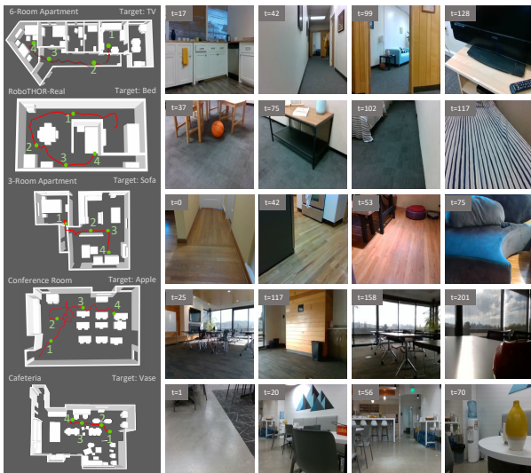
Figure 8. Qualitative results. These demonstrate the ability of PHONE2PROC models to navigate to their desired object. The top-down map is for visualization purposes only and is an approximation of the path taken by the agent.
