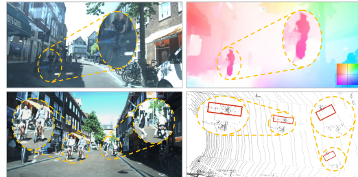
Figure 3. Illustration of the causes of noisy supervision signals from camera and LiDAR. The top row shows an example of the noisy optical flow estimation on RGB images. The bottom row exhibits unreliable object recognition on LiDAR point clouds. We enlarge regions of interest and mark them with amber circles.
