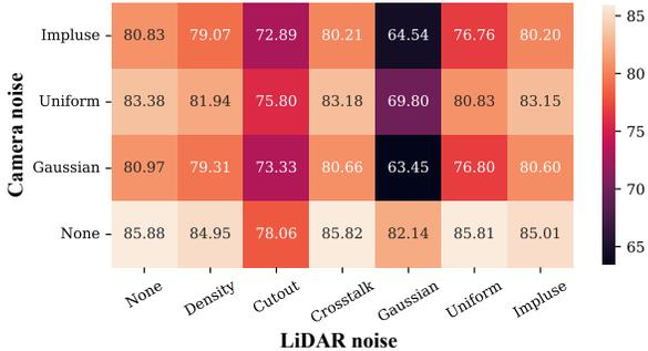
Figure 4. The performance of Focals Conv [13] under the concurrence of LiDAR and camera noises.
