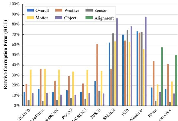
Figure 3. The relative corruption error RCE of 11 3D object detectors on **KITTI-C**. We show the overall results under all corruptions and the results under each level of corruptions.
