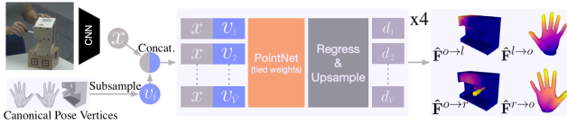
Figure 6. InterField-SF architecture. We concatenate image features \mathbf{x} to each subsampled hand-object vertex in canonical pose. The concatenated vectors are passed through a PointNet and then regressed to distance values. The interaction field is visualized as a heatmap for each entity (bright: closest vertex is near).
