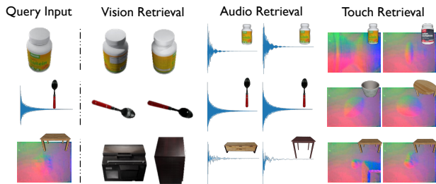
Figure 3. Examples of the top-2 retrieved instances for each modality using DAR [2], the best-performing baseline. For audio and touch retrieval, we also show an image of the object.
