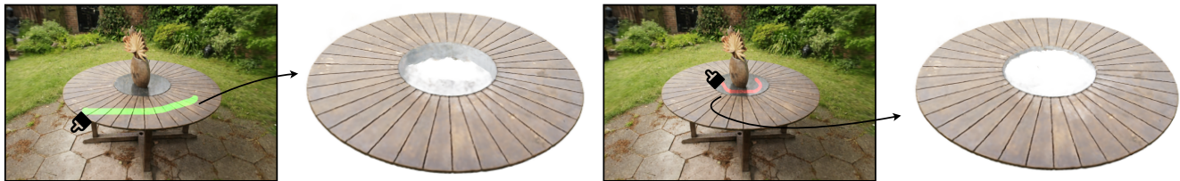
Figure 1. We present ISRF, an interactive method to segment objects in radiance fields. Users can draw positive strokes to segment multiple objects at a time in 3D and negative strokes to remove unwanted regions repeatedly. In the figure, the WOODEN TABLE TOP is segmented using one positive and one negative stroke as shown.
