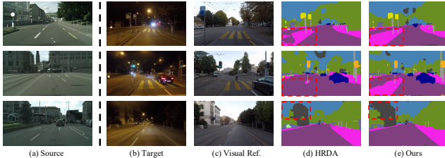
Figure 4. Qualitative Comparisons for UDA Semantic Segmentation, under Cityscapes → Dark Zurich. (a) shows the example of Cityscapes images. (b) includes the Dark Zurich images. (c) covers the day images corresponding to the night images in (b) for better visual references. Note that, the day images in (c) are only used for visualization references, but are not used for training and testing. (d) and (e) are the segmentation results for (b) from HRDA [24] and our method, respectively.
