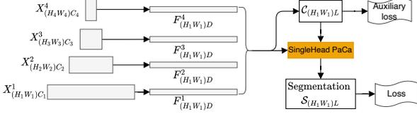
Figure 5. The proposed PaCa head network for semantic segmentation. The feature pyramid from the backbone (Fig. 3) is projected to a  $D$ -dim feature space and resized to the resolution of the first feature layer (via bilinear interpolation).  $L$  is the number of classes (e.g., 150 in the MIT-ADE20k dataset). Both the losses are cross-entropy, but with a smaller weight for the auxiliary loss.
