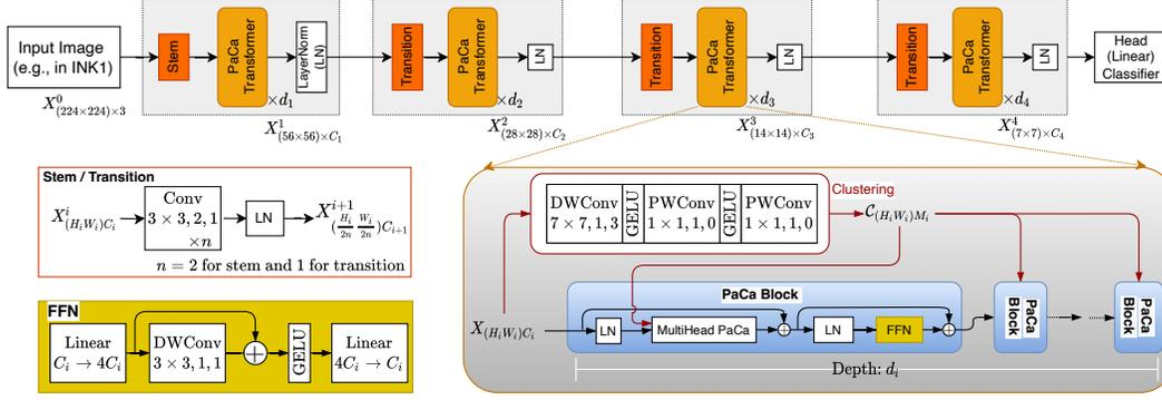
Figure 3. Illustration of the proposed PaCa-ViT using the stage-wise convolution-based clustering setting. It consists of four stages each of which has a number,  $d_i$  of the proposed PaCa Transformer block. The FFN refers to a feed-forward network. See text for details.
