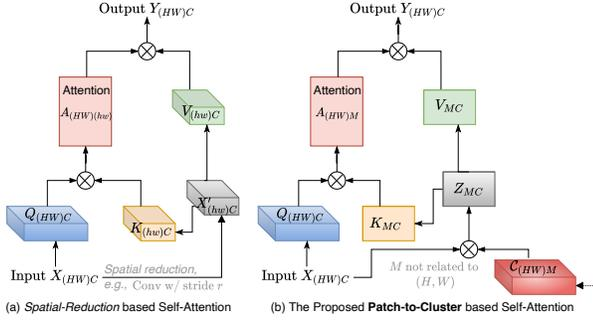
Figure 2. Illustration of (a) the spatial reduction based self-attention and (b) the proposed PaCa module in vision applications, where  $(HW)$  represents the number of patches in the input with  $H$  and  $W$  the height and width respectively, and  $M$  a predefined small number of clusters (e.g.,  $M = 100$ ). See text for details.
