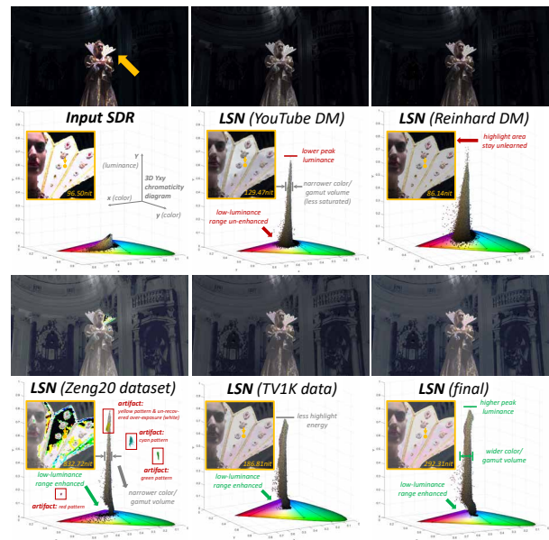
Figure 8. Result of ablation studies proves the importance of both high-quality label HDR and rational DMs. Specifically, absent of both label HDR’s HDR/WCG volume (Zeng20) and DM’s degradation ( Reinhard ) will impair LSN’s recover ability, meanwhile YouTube DM’s style will make our LSN commonplace as others.
