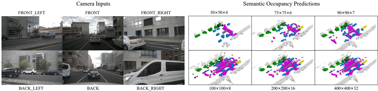
Figure 6. **Arbitrary resolution at test time.** We can adjust the prediction resolution through interpolation at test time.
