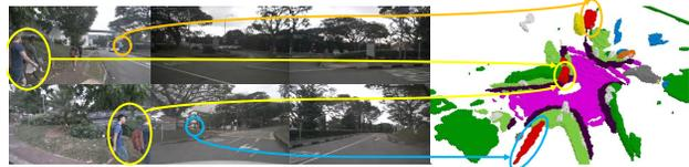
Figure 7. Failure cases of pedestrians for semantic occupancy prediction. TPVFormer has trouble distinguishing pedestrians close to each other and could predict a strip area for a distant pedestrian. the comparable latency of TPV and voxel.
