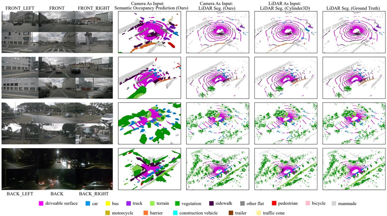
Figure 5. **Visualization results on 3D semantic occupancy prediction and nuScenes LiDAR segmentation.** Our method can generate more comprehensive prediction results than the LiDAR segmentation ground truth.
