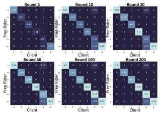
Figure 4. Free rider study. Each row denotes an independent federated training procedure, and the y-axis indicates which client is the free rider. A free rider is detected with a high value.
