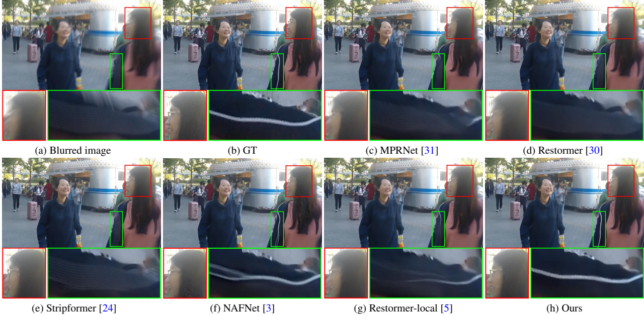
Figure 5. Deblurred results on the HIDE dataset [20]. The deblurred results in (c)-(g) still contain significant blur effects. The proposed method generates much clearer images.
