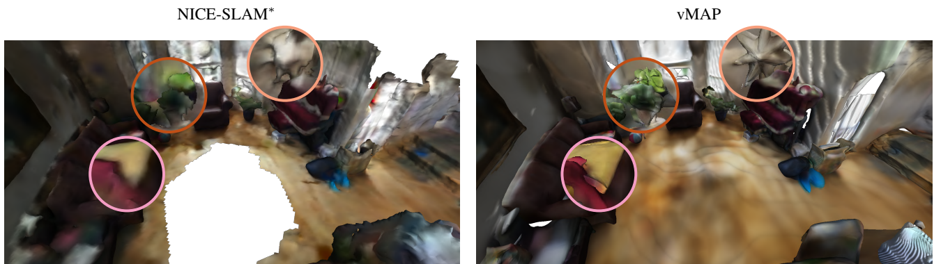
Figure 5. Visualisation of scene reconstruction from NICE-SLAM* (left) and vMAP (right) in a selected ScanNet sequence. Interesting regions are zoomed in. NICE-SLAM* was re-trained with ground-truth poses.
