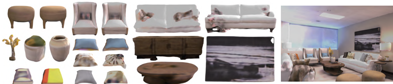
Figure 1. vMAP automatically builds an object-level scene model from a real-time RGB-D input stream. Each object is represented by a separate MLP neural field model, all optimised in parallel via vectorised training. We use no 3D shape priors, but the MLP representation encourages object reconstruction to be watertight and complete, even when objects are partially observed or are heavily occluded in the input images. See for instance the separate reconstructions of the armchairs, sofas and cushions, which were mutually occluding each other, in this example from Replica.
