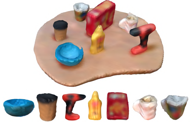
Figure 7. Visualisation of table-top reconstruction (top) and individual object reconstructions (bottom), from vMAP running in real time using an Azure Kinect RGB-D camera for 170 seconds.
