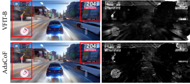
Figure 3. Visualization of Discontinuity map ( D -map) estimated for a sample. AdaCoF and VFIT-B are the baseline networks where we apply our methods. D -map commonly shows the user interface elements (UI) that are fixed on their position and some digits that change dynamically (highlighted in red boxes).
