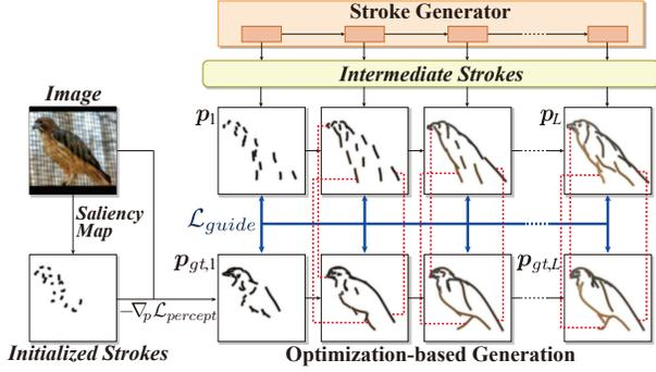
Figure 4. Visualization of the progressive optimization process. Strokes initialized from the saliency map are optimized using the gradient of  $\mathcal{L}_{percept}$  until convergence and stored in a total of  $L$  intermediate steps denoted by  $p_{gt,l}$ . Then, the stroke generator is trained through  $\mathcal{L}_{guide}$  to progressively predict each intermediate stroke  $p_l$  from  $p_{gt,l}$ .
