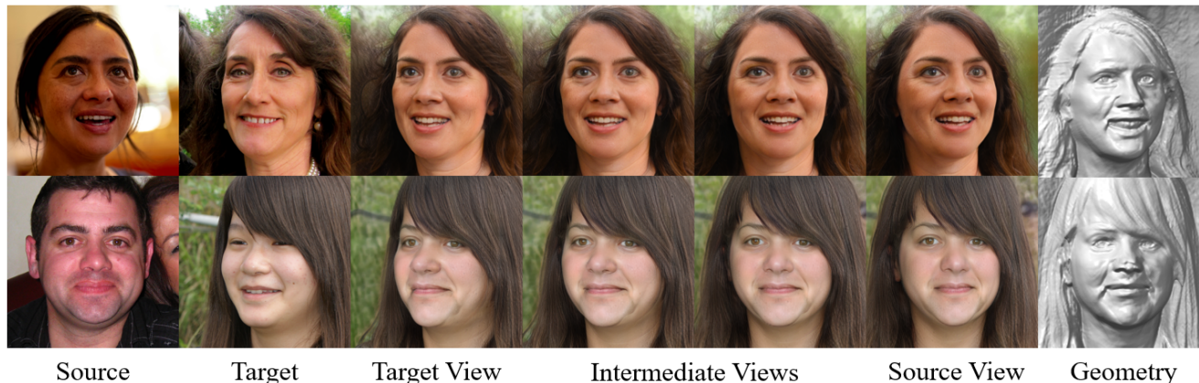
Figure 1. Demonstration of the proposed 3dSwap. Given single-view source and target images, our method synthesizes high-fidelity and multi-view-consistent images of the swapped faces and the corresponding geometries. More results can be found on our project page.
