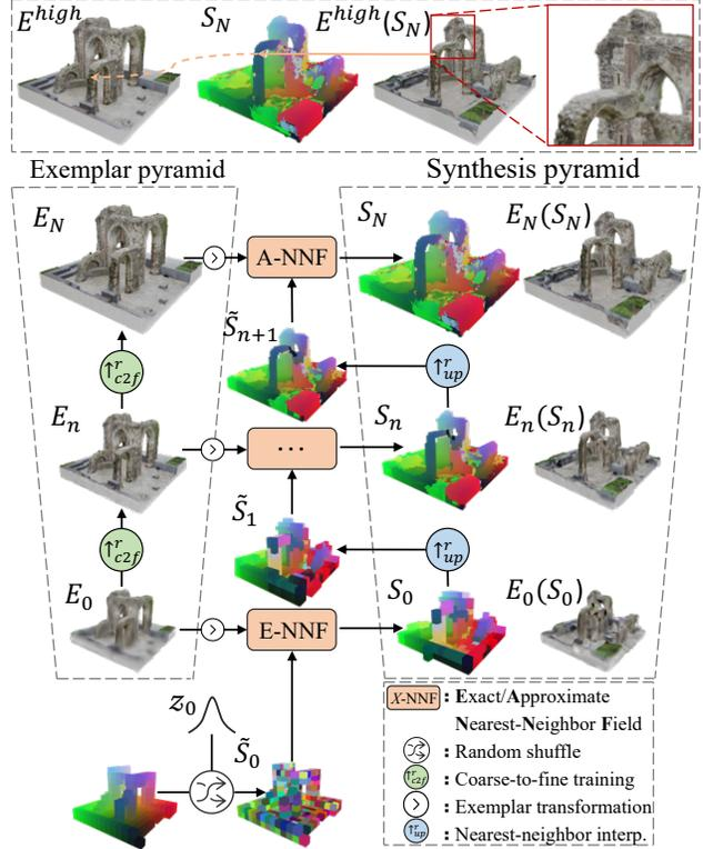
Figure 3. Multi-scale generation. At each scale  $n$ , the NNF module updates the generation based on the transformed exemplar  $\hat{E}_n$  and an initial guess  $\tilde{S}_n$  upscaled from the previous. The coarsest scale takes a shuffled identity mapping field as input. Note that our coordinate-based representation  $S_N$  can map to patches in a higher-resolution exemplar for higher quality (top row).
