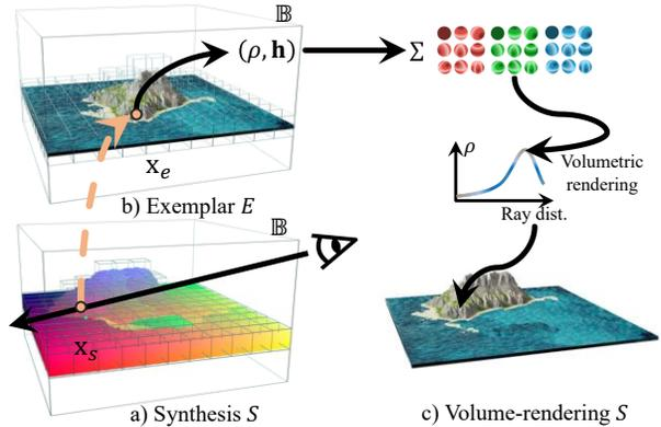
Figure 2. a) The synthesized scene  $S$  is represented as a field mapping a coordinate in  $S$  to one in  $E$ . b) The Plenoxels-based exemplar  $E$  uses a sparse grid, where each occupied voxel stores a scalar opacity  $\rho$  and spherical harmonic coefficients  $\mathbf{h}$ . c) Appealing imagery of  $S$  can be produced via the volumetric rendering function. Empty voxels are omitted for simplicity.
