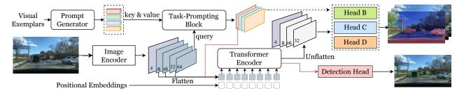
Figure 3. The architecture of the proposed VE-Prompt. VE-Prompt consists of (1) the image encoder to extract image features; (2) a shared transformer encoder for feature enhancement; (3) task-specific prompts generated by the prompt generator with visual exemplars; (4) a task-prompting block to integrate the visual representation with task-specific prompts; and (5) task-specific heads for different tasks.
