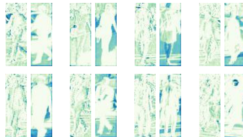
Figure 3. We compare the feature maps extracted by the model without (left) and the model with DFF (right). The lighter the color is, the larger the feature value is.
