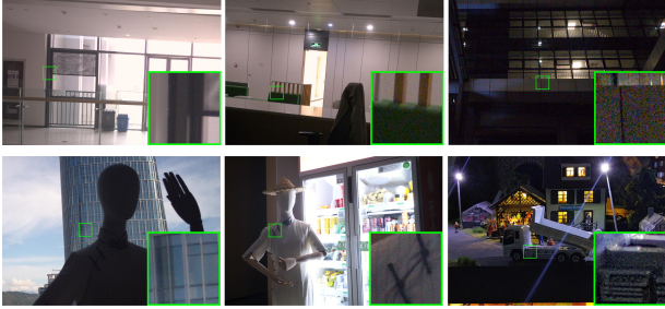
Figure 2. Sample LDR frames in our Mobile-HDR dataset. Various noise levels can be observed in the zoomed-in regions. The images are visualized through a simple ISP pipeline.
