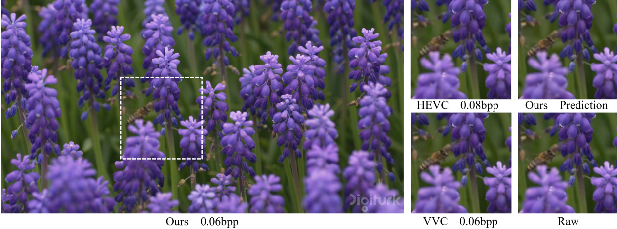
Figure 2. Reconstruction with standard codecs (HEVC, VVC) and our MMVC method. Details of the static background and dynamic objects are well preserved in the frame generated from the predicted features and entropy-coded residuals that are block wise selected from multiple modes. Compared with HEVC, our result yields less block artifacts preserving finer details. Our method achieves high quality similar to that of VVC codec, which is the state-of-the-art standard released recently.
