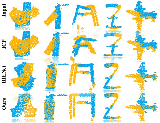
Figure 5. Registration results of different methods on ModelLoNet with more than 50% partial overlaps.
