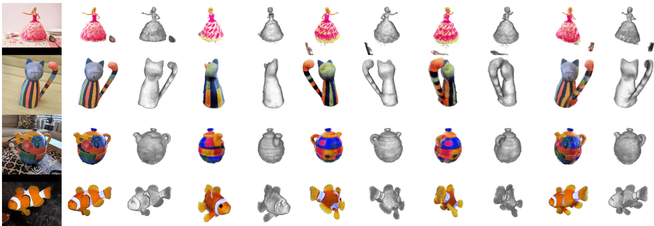
Figure 1. RealFusion generates a full 360° reconstruction of any object given a single image of it (left column). It does so by leveraging an existing diffusion-based 2D image generator. From the given image, it synthesizes a prompt that causes the diffusion model to “dream up” other views of the object. It then extracts a neural radiance field from the original image and the diffusion model-based prior, thereby reconstructing the object in full. Both appearance and geometry are reconstructed faithfully and extrapolated in a plausible manner.
