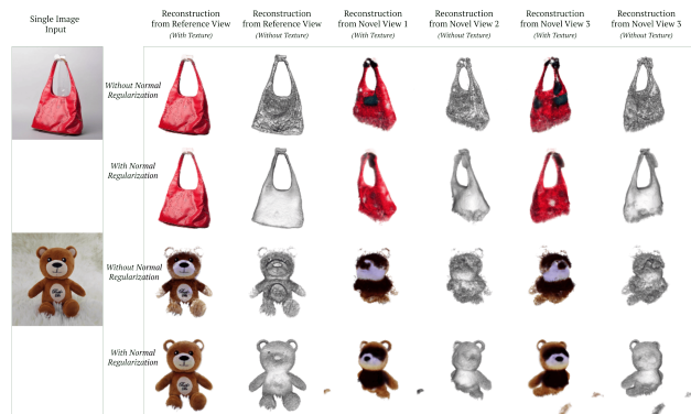
Figure 9. Effect of normal smoothness on reconstruction quality. Each pair of rows show the reconstruction without and with the normal smoothness regularization term (4). The regularizer improves the visual appearance of surfaces and reduces the number of irregularities on the surface of reconstructed objects. In most cases, we also find that it helps to improve the overall realism of the reconstructed shape.
