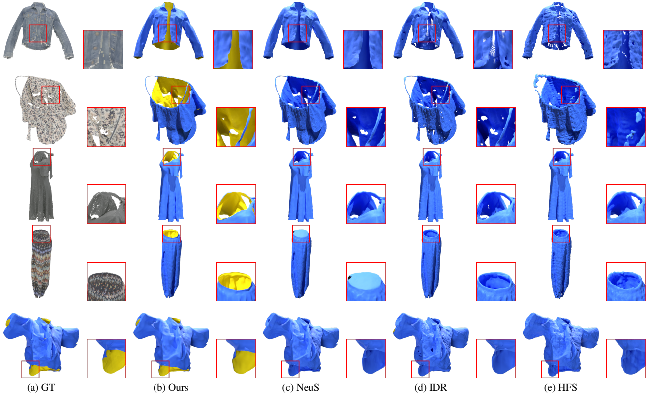
Figure 7. Comparisons on open surface reconstruction. Row 1 – 4 are evaluated on Deep Fashion 3D Dataset [19] and Row 5 is evaluated on Multi-Garment Net Dataset [4]. NeAT is able to reconstruct high-fidelity open surfaces while NeuS [48], IDR [55] and HFS [49] fail to recover the correct topologies.
