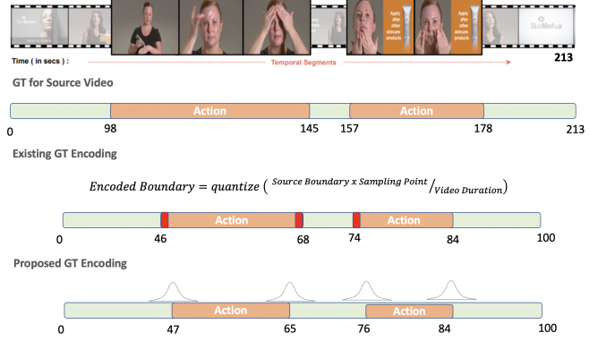
Figure 6. Illustration of quantization error in the standard ground-truth (GT) generation: Obtaining the start/end points with floor based snippet quantization. As a result, an error (indicated by red marker) is introduced. Other quantization (e.g., ceiling, rounding) share the same problem.
