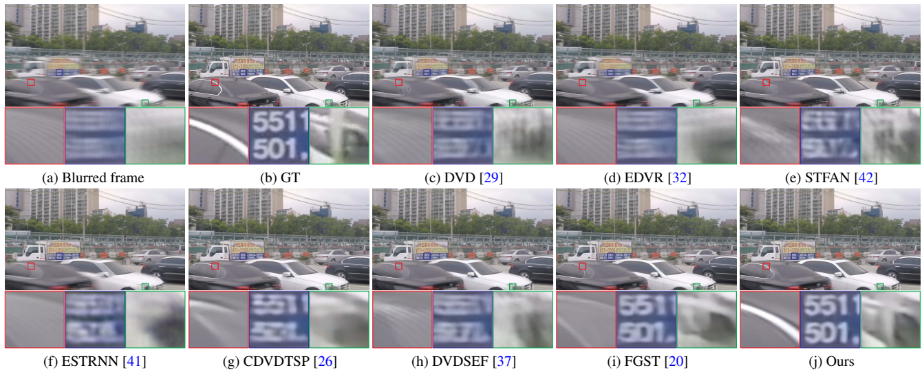
Figure 4. Deblurred results on the GoPro dataset [24]. The deblurred results in (c)-(i) still contain significant blur effects. The proposed method generates much clearer frames.
