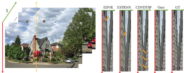
Figure 9. Visual comparisons of the temporal consistency for restored videos. We visualize the pixels of the selected columns (the dotted line) according to [4].
