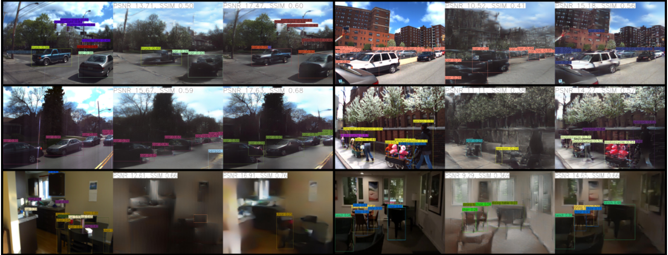
Figure 2. Left to right: original image, reconstructions from SegLoc and PixLoc 3D models. We also show the yolov7 detections.
