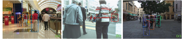
Figure 6. Visualization of Directed Interaction. The boxes in different colors represent the bounding boxes of different targets, the end of arrow represents the affecting target, and the head of arrow represents affected target.
