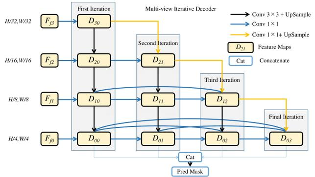
Figure 6. The structure of our Multi-view Iterative Decoder. It mimics the process people do careful analysis and utilizes the encoder’s output features in different resolution iteratively to find out subtle tampering clues.
