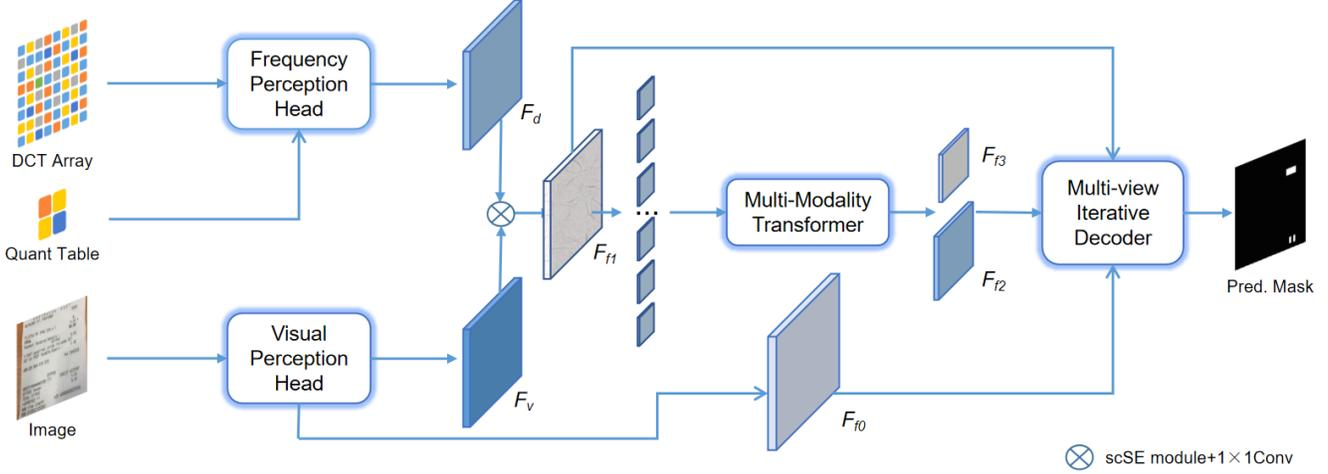
Figure 4. The overall architecture of our model. We extract visual domain features from image with Visual Perception Head and extract frequency domain features from DCT coefficients with Frequency Perception Head. Then fuse them and extract multi-modality features by multi-modality Transformer. At last, we utilize Multi-view Iterative Decoder to get predictions with encoder’s output features.
