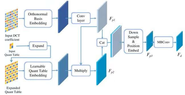
Figure 5. The structure of our Frequency Perception Head. It takes DCT coefficients with the quantization table of the image  $I$  as input, and outputs frequency feature embeddings.
