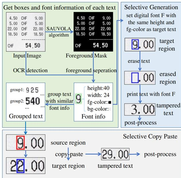
Figure 3. The pipeline of the proposed data synthesis method. We first record size, foreground color and background color of each text and then do selective synthesis based on that.
