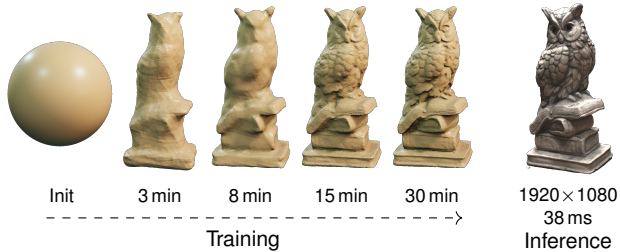
Figure 4. We train for 30 min using posed images and afterwards render novel views in real-time using sphere tracing.
