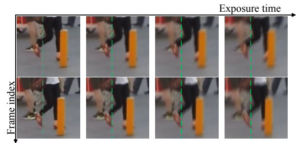
Figure 1. Visualization of motion blur under different exposure time and object motion. Frames from the left to right are obtained with increasing exposure time, leading to severer degree of motion blur. The situation may be worse if stronger motion is present, as illustrated by images in the second row.
