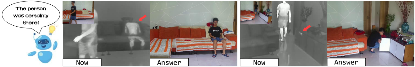
Figure 2. Thermal images to the rescue: Thermal images encode traces of past human-object interactions, which can help us infer past human behavior and understand objects’ affordance. In this work, we focus on estimating human body poses a few seconds ago.
