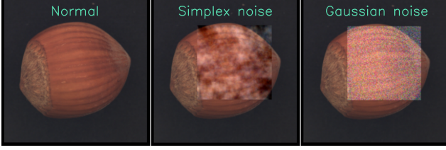
Figure 3. Comparison between Simplex noise [37] and Gaussian noise in simulating the pseudo-anomalous regions in the image. Simplex noise generates a more natural pseudo-anomaly.
