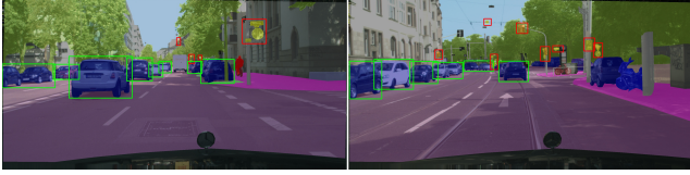
Figure 2. Illustration of the Presence of Classes between Major (green boxes) and Minor (red boxes) Groups. Classes in the minority group typically occupy fewer pixels than the ones in the majority group (Best view in color and 2× zoom).
