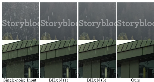
Figure 6. Visual comparisons for real-world rainstreak removal on SPADData [52] for task II. BIDeN(1) means a two-head network trained with a single-type rainstreak mask and BIDeN(3) means the four-head structure trained with rainstreak + raindrop + snow.
