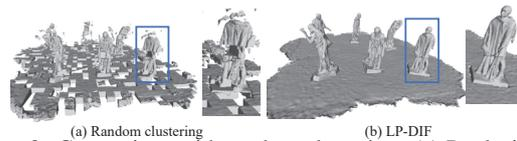
Figure 8. Comparison with random clustering. (a) Replacing the clustering process with random assigning each local region into clusters. (b) Clustering with regards to similarity leads to better performance.
