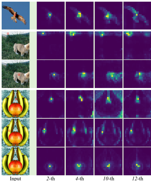
Figure 4. Visualization of the attention maps for different query points, marked with red boxes. LocalMIM can distinguish semantic regions using self-attention mechanism.
