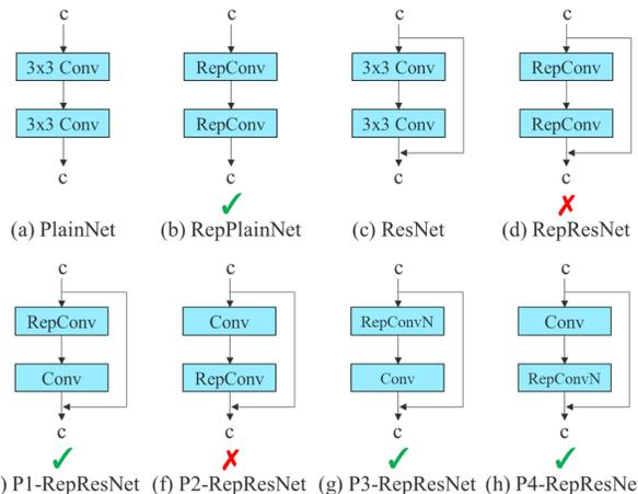
Figure 4. Planned re-parameterization model. In the proposed planned re-parameterization model, we found that a layer with residual or concatenation connections, its RepConv should not have identity connection. Under these circumstances, it can be replaced by RepConvN that contains no identity connections.
