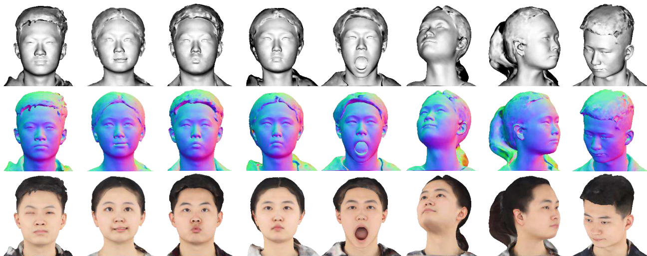
Figure 1. We propose GANHead to generate diverse head avatars with complete geometry and realistic texture. The generated avatars can be deformed to target poses and expressions through FLAME [22] parameters, which generalize well to unseen poses and expressions.
