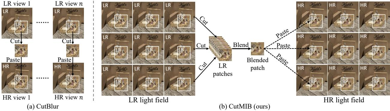
Figure 2. Illustrative examples of (a) CutBlur and (b) our proposed CutMIB. CutBlur generates augmented SAIs view-by-view via the “cutting-pasting” operation. CutMIB generates the augmented light field via the “cutting-blending-pasting” operation. The implicit geometric information can be utilized during the training stage.
