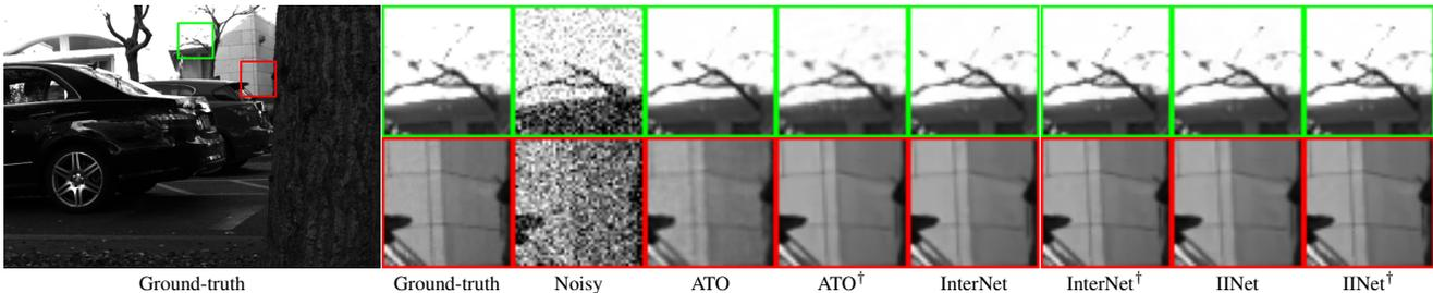
Figure 8. Visual comparisons (view coordinates: (4, 4) in an  $8 \times 8$  light field) of different models trained without and with the proposed CutMIB on light field denoising under the setting of  $\sigma = 50$ . Please zoom in for better visualization and best viewed on the screen.
