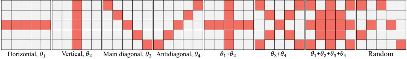
Figure 5. Variants of CutMIB on a light field with  $5 \times 5$  angular resolution. Red rectangles denote the views in a light field utilized in CutMIB (*i.e.*, the cutting-blending-pasting operations). Gray rectangles denote the views trained without the CutMIB strategy.
