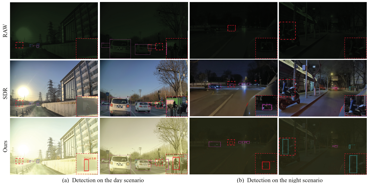
Figure 5. Visual examples of object detection. (a) and (b) are detection results on the day and night scenarios of the ROD dataset, respectively. From top to bottom are the results of RAW data, SDR data, and our method, respectively. Our method significantly outperforms the SDR data. Please zoom in for confidence scores and class predictions. More visual results are in the supplementary document.
