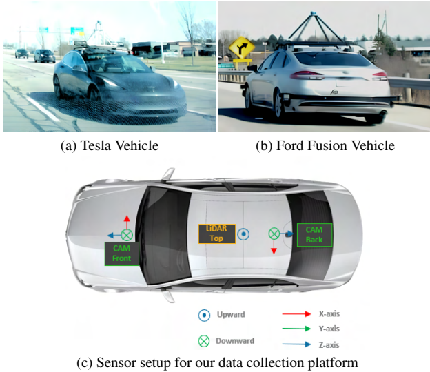
Figure 2. The information of the collection vehicles. a) The Tesla vehicle. b) The Ford Fusion vehicle. c) The sensor setup for both vehicles. Note that the photo of Tesla is taken from the rear camera of Ford, and that of Ford is taken from the front camera of Tesla.
