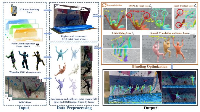
Figure 4. **Overview of main annotation pipeline.** The blue arrows indicate data flows, and the yellow arrows represent the direction of optimization. **Dotted box:** The input of each scene consists of RGB videos, point cloud sequence, IMU measurements, and 3D laser scanning data. Data pre-processing stage calibrates and synchronizes different modalities. **Solid box:** The blending optimization stage optimize including the pose and translation based on multiple constraint losses.
