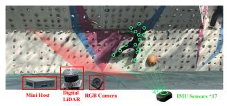
Figure 3. **Data Capturing System.** Including 17 wearable IMU sensors, a LiDAR, a RGB camera and a computer.
