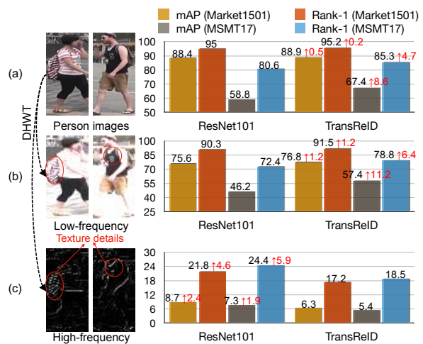
Figure 1. Performance comparisons between ResNet101 ( 44.7M #Param ) and TransReID ( 100M #Param ) on (a) original person images, (b) low-frequency components, and (c) high-frequency components of Market1501 and MSMT17 datasets, respectively. Note that “#Param” refers to the number of parameters.
